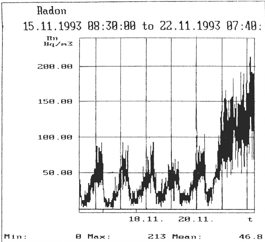
Figure 1. Variation in Radon levels over seven days.
