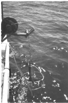
Cover Picture: Deployment of ICTD probe for profiles of sea temperature and salinity.
