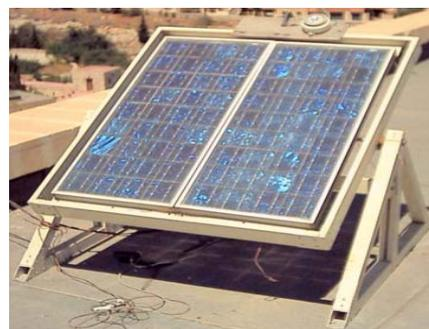
Figure 6 Polycrystalline solar panels and pyranometer.
