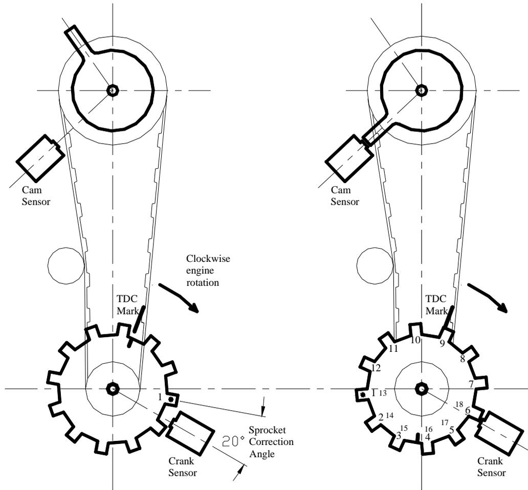
**Figure 13 Case 1, Left: Determination of Sprocket Correction Angle and Tooth No 1, Right: Determination of Tooth at Cam Sensor**
