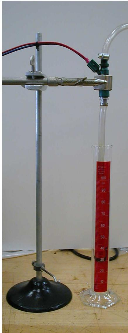
**Figure 1 Injector Flow Test**
