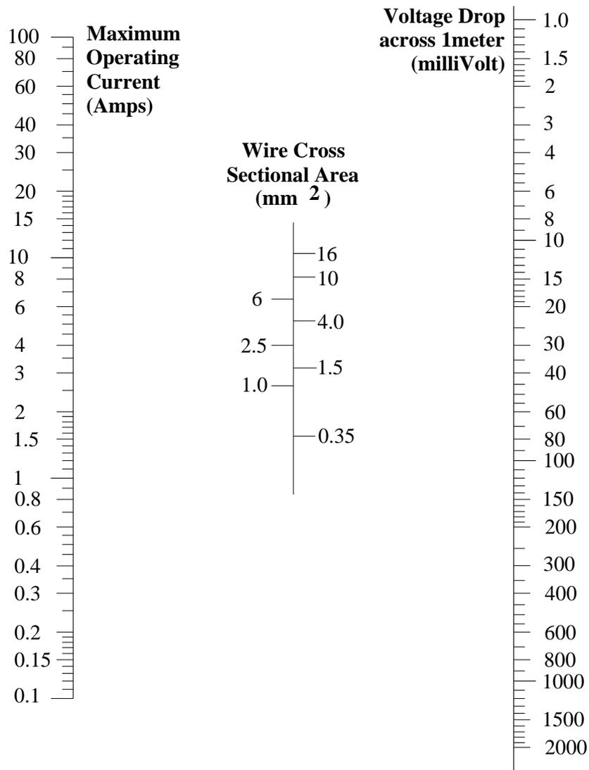
Figure 19 Wire Cross-sectional Area Nomogram
