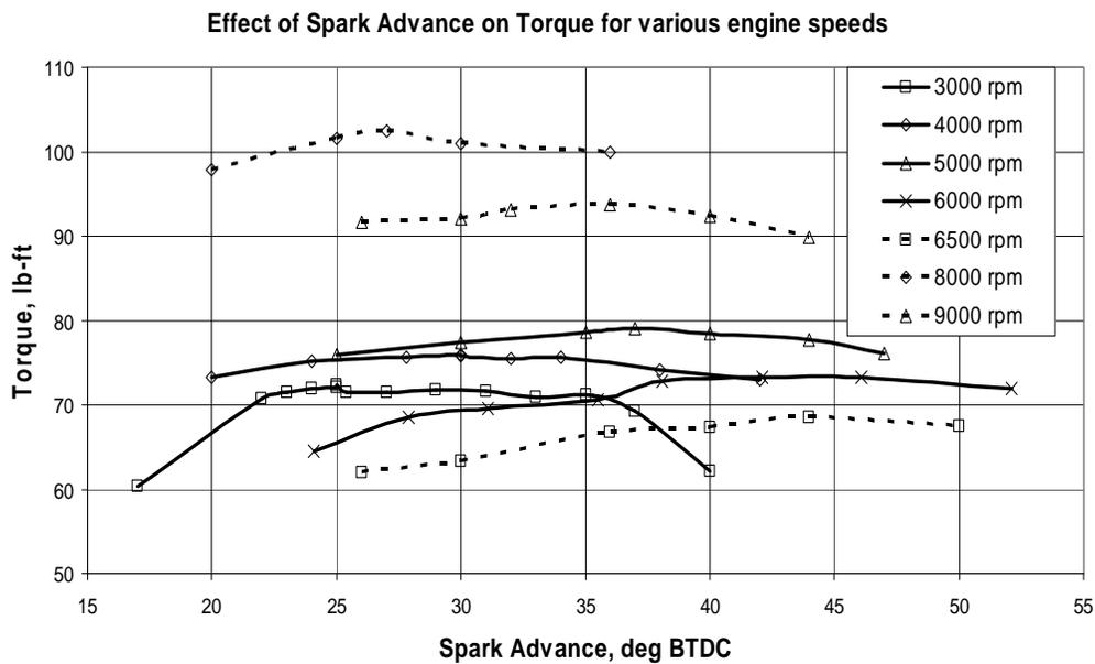
**Figure 4 Spark Advance Hooks at WOT**
