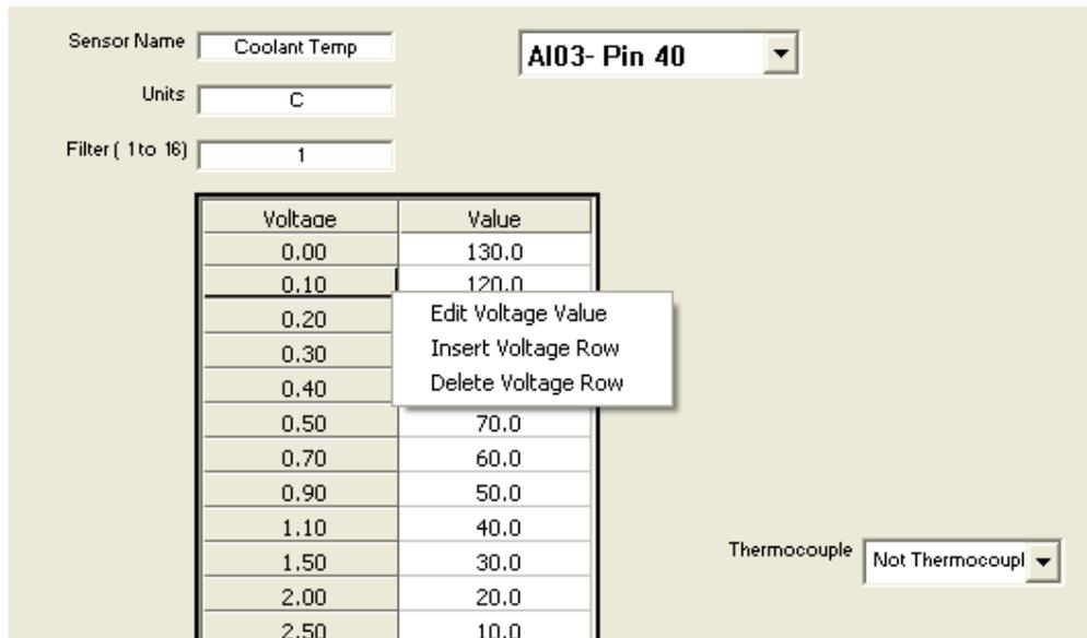
**Figure 7 Setting the Voltage entries in Sensor Conversion**
