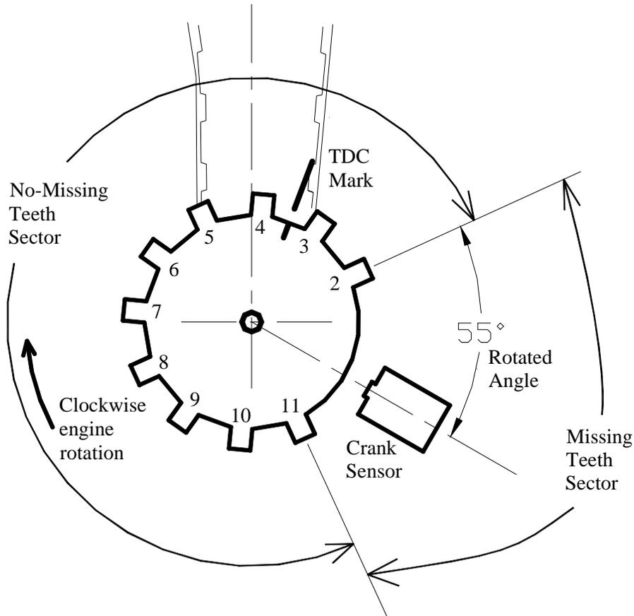
**Figure 15 Case 2B, Determination of Sprocket Correction Angle and Last Non-Missing Tooth on Crank Sprocket**
