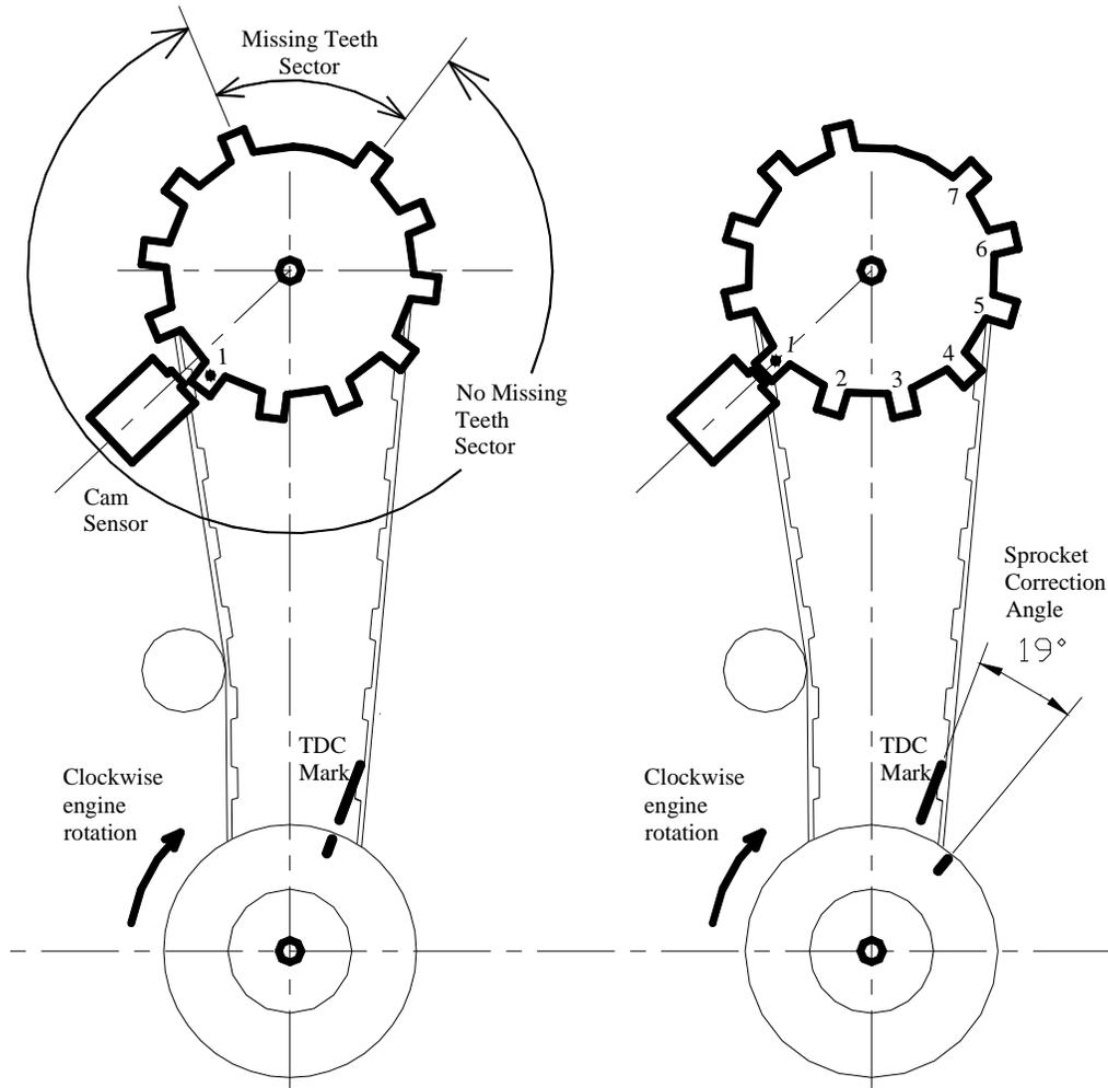
**Figure 16 Case 3A, Determination of Sprocket Correction Angle and Last Non-Missing Tooth on Cam Sprocket**
