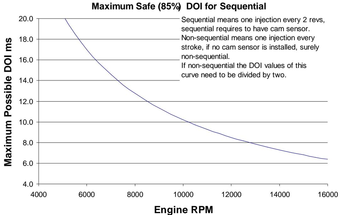
**Figure 9 Maximum Injector DOI as a function of engine RPM, sequential & 85% factor**
