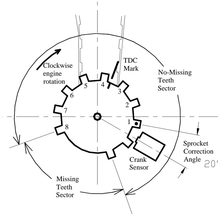
**Figure 14 Case 2A, Determination of Sprocket Correction Angle and Last Non-Missing Tooth on Crank Sprocket**
