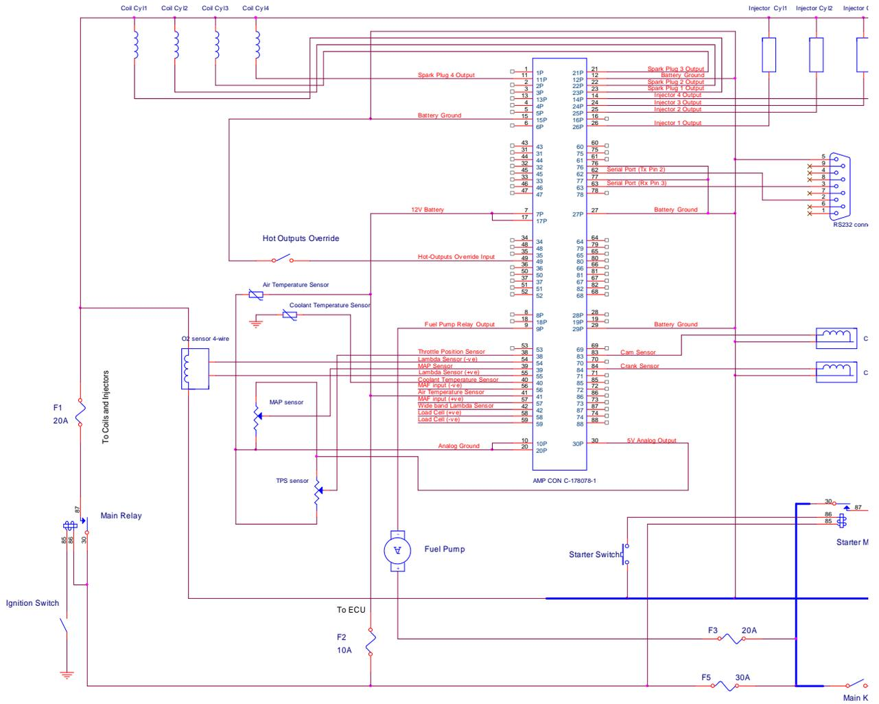
Figure 18 Basic Harness Wiring Setup
