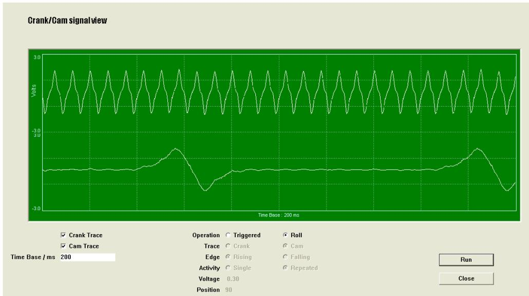
Figure 8 Oscilloscope View Dialogue
