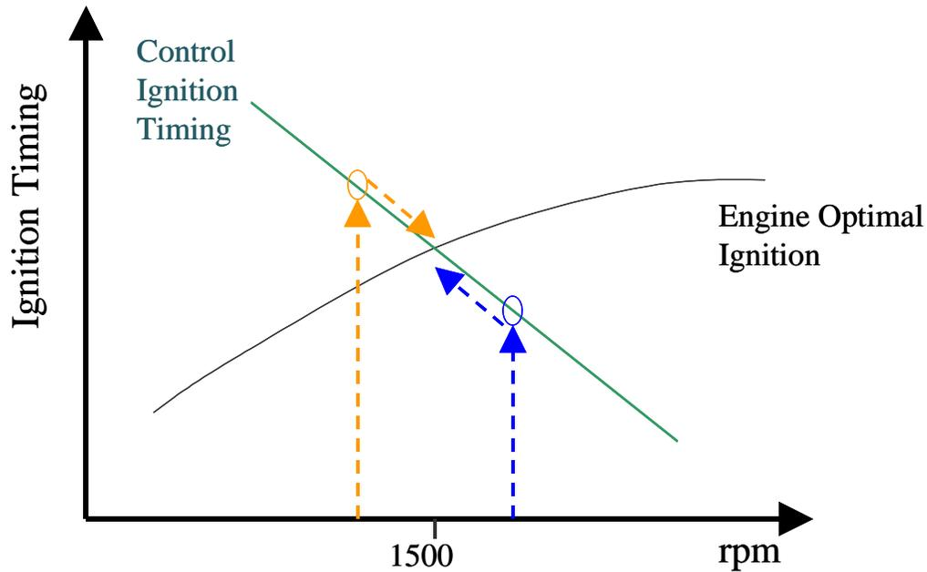
**Figure 10 Idle Speed Control Strategy, without idle speed control motor**
