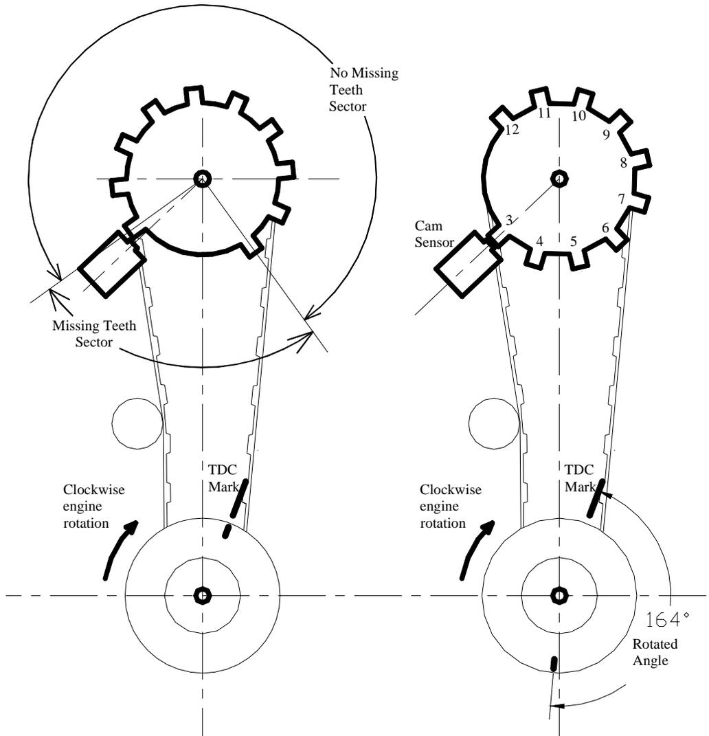
**Figure 17 Case 3B, Determination of Sprocket Correction Angle and Last Non-Missing Tooth on Cam Sprocket**
