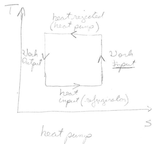
For such a heat pump the set up would be
