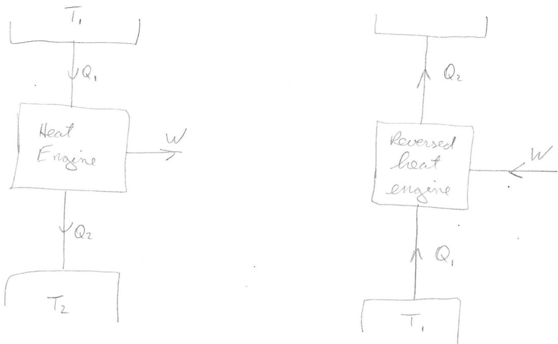
By the First Law of Thermodynamics for the Reversed heat engine
