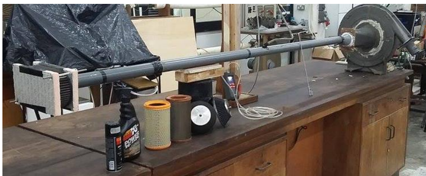
Figure 4: The air filterflow test setup
