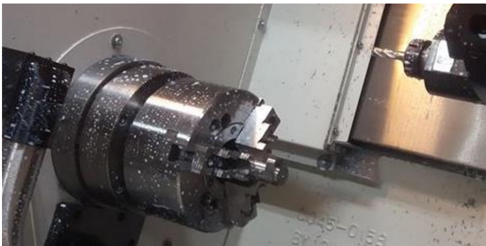
Figure 15: The camshaft being manufactured on a 3-axis CNC lathe
