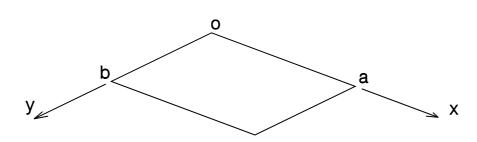
Using an energy method find the transverse displacement w anywhere along the plate. The deflected form of the plate may be assumed to be  $w = \sum_{m=1}^{\infty} \sum_{n=1}^{\infty} A_{mn} \sin \frac{m \pi x}{a} \sin \frac{n \pi y}{b}$ .
