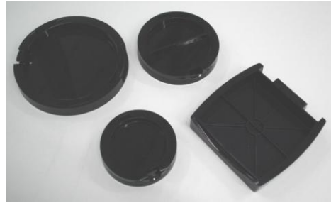
Figure 4 - A range of the different shapes and sizes of base containers to be handled. Colour and reflectivity also vary.
