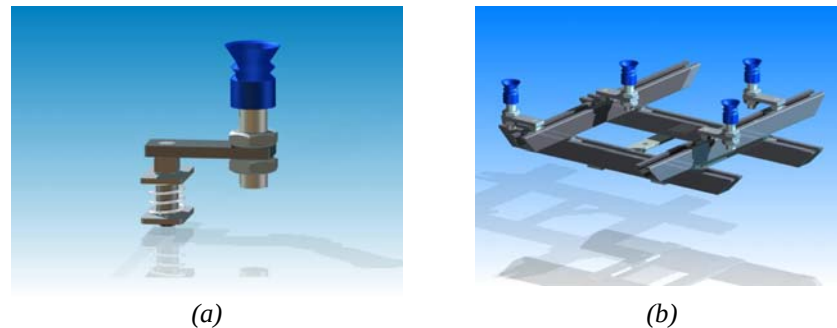
Figure 5: (a) gripper fixture design, (b) reconfigurable rail design
