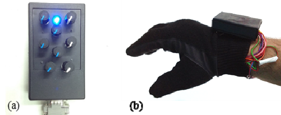
Figure 8. (a) Handheld input device containing eight potentiometers; (b) Glove input device containing eight flexible bend sensors
