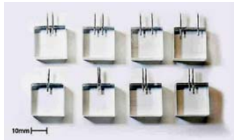
Figure 3. The two point discrimination test apparatus
