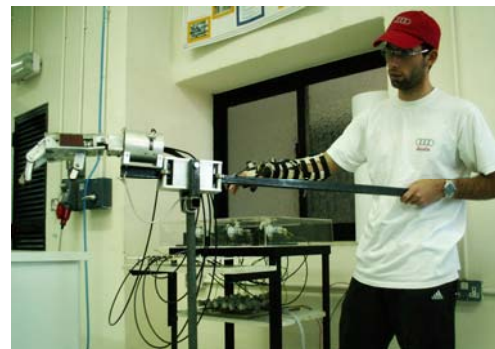
Fig. 17. The anthropomorphic robot hand and wrist, mounted on the metal stand and teleoperated using the glove input device.
