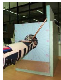
Figure 12. Testing of angular position measurement for forearm roll.
