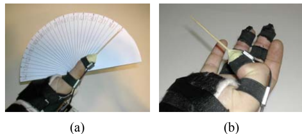
Figure 10. Testing of angular position measurement for thumb, (a) fully extended, and (b) fully flexed (position template not shown).
