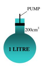
7 A pump is used to exhaust a vessel of volume 1 litre containing air at 1.2 atmospheres, at constant temperature. The pump has an effective volume of  $200 \text{cm}^3$  and at each stroke this volume of air is expelled to the atmosphere.
