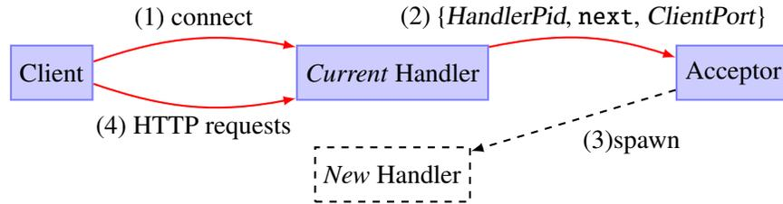
Figure 1: Yaws client connection protocol
