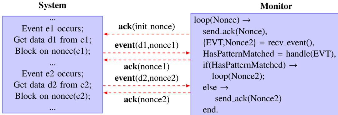
Figure 4: A high level description of the synchronous event monitoring protocol.
